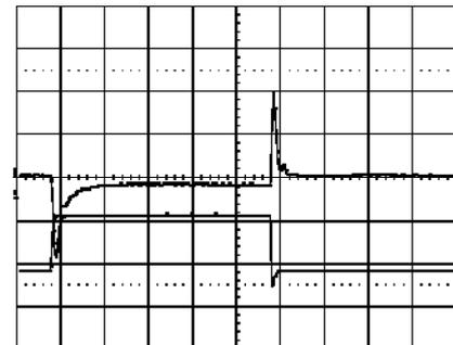
Output voltage response to load current step- Trace: output voltage (100mV/div.).
