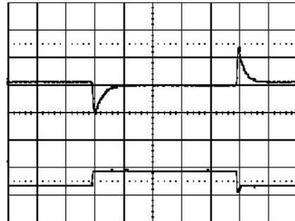
Output voltage response to load current step- Trace: output voltage (200mV/div.).
