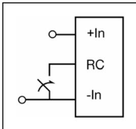
The products are fitted with a remote control function referenced to the primary negative input connection (- In), with negative and positive logic options available. The RC function allows the converter to be turned on/off by an external device like a semiconductor or mechanical switch.
