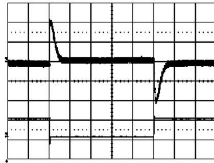
Output voltage response to load current step-
