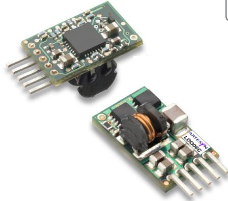
The LDO06C series is a new high density, open frame, non-isolated converter for space sensitive applications. This model has a wide input range of 3-13.8 V and offers a 0.59-5.1 V adjustable output with 6 A capability. Typical efficiency for this model is 92% (5 Vin, 2.5 Vout, 6 A load). The 5 pin version of this voltage device offers the standard features of enable, and with a default wide adjustable output voltage range or option of power good.
