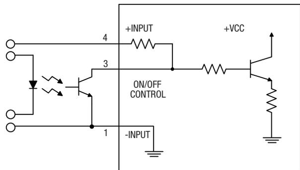
Figure C. Driving the On/Off Control Pin (suggested circuit)
