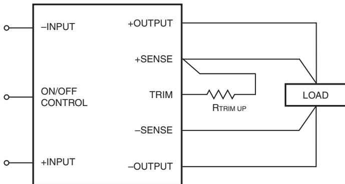
Figure B. Trim Connections To Increase Output Voltages
