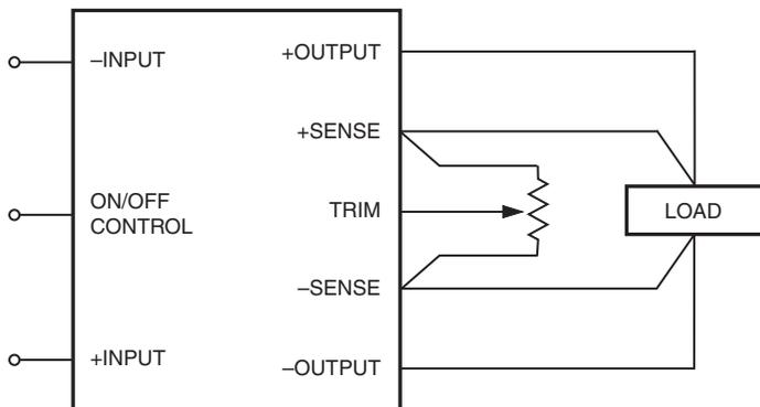
Figure A. Trim Connections Using A Trimpot
