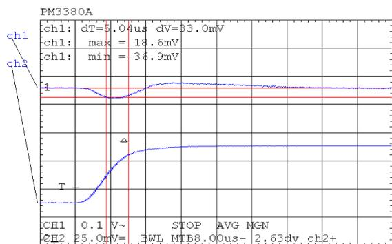
$V_{IN} = 4.0V_{DC}$   $V_{OUT} = 3.3V_{DC}$   $I_{OUT}$  Change = 100-50%
