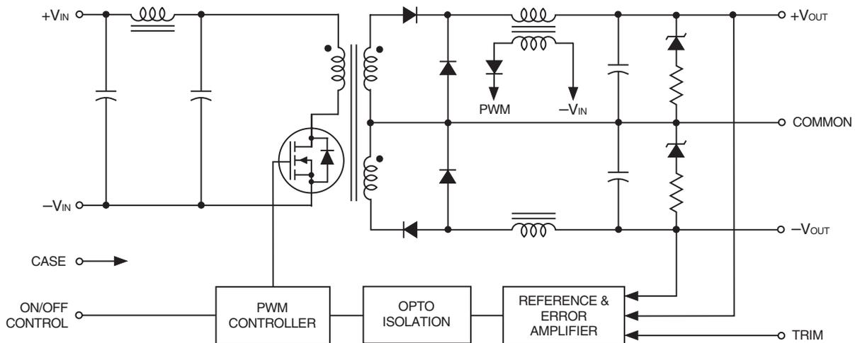
Figure 1. Simplified Schematic
