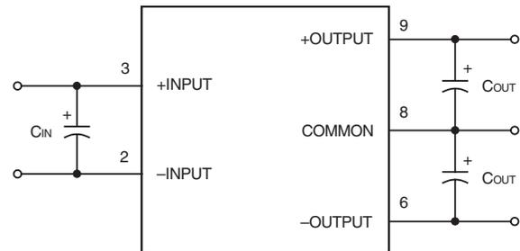
Figure 7. Using External Capacitors to Reduce Input/Output Ripple/Noise
